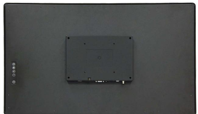
faytech's Capacitive Touch Monitors have a modern sleek look with its flat edge to edge glass IP65 water- and dust proof front panels. This device has capacitive 10-finger multitouch, glass front reaching MosH 7, the glass surface is anti-glare treated (chemical etching) and a wide variety of connectors. All the monitors have VESA 75 or VESA 100 screw patterns on the back, while the 13.3" to 27" come with their own desktop stand included.
